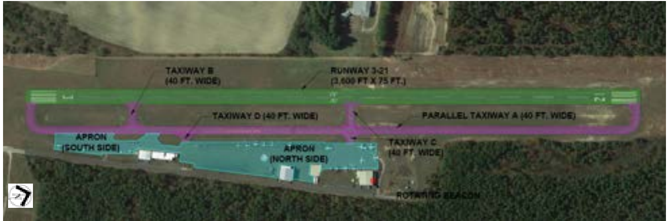
Figure 1-2 Existing Airside Facilities
